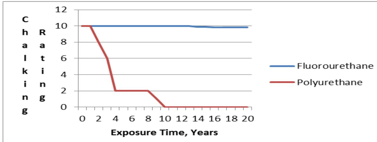
In the chalking test, topcoat properties are monitored over time. Chalking (coating degradation by UV light and corrosives) is rated from 0-10, with 10 being no chalking and 0 being severe chalking over the entire coating surface. The performance of FEVE fluoropolymer compared to polyurethane is striking.
